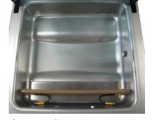
SEALING BAR 16,5 inch VACUUM PUMP 883 cf/h SENSOR CONTROL
